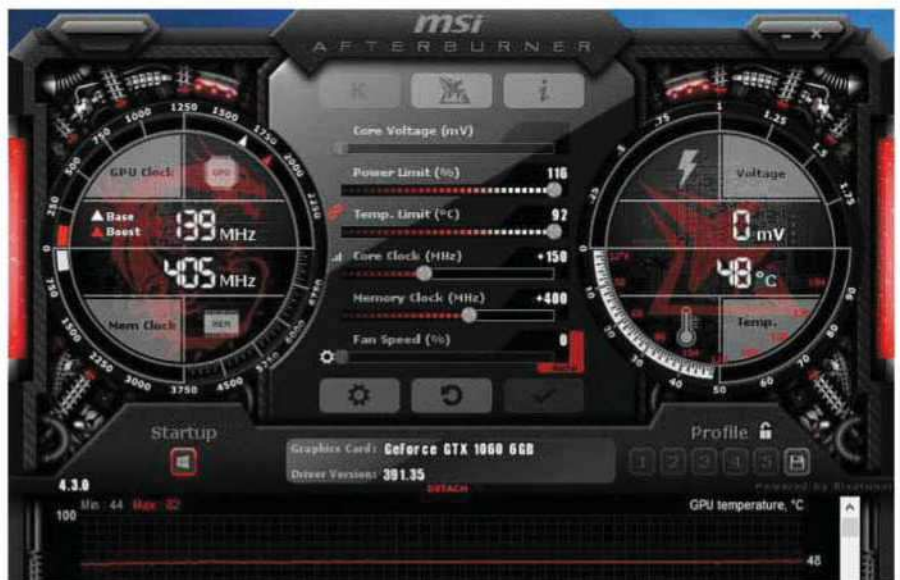
Add 150MHz to the core clock and 400MHz to the memory clock in MSI Afterburner
