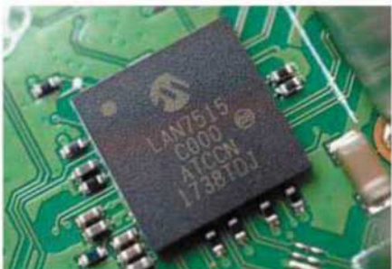
The new Ethernet and USB controller provides a Gigabit Ethernet connection, but sadly not Gigabit throughput
