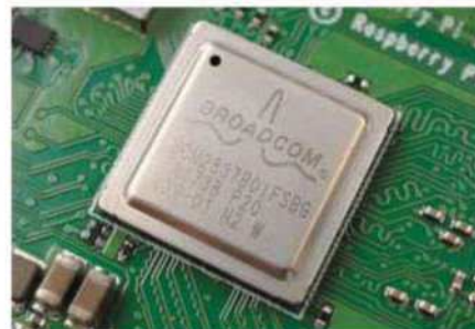
New packaging and bonding has improved the thermal characteristics of the BCM2837 SoC considerably
