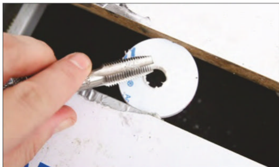
Tapping thick materials manually can be tough, even in soft materials such as acrylic
