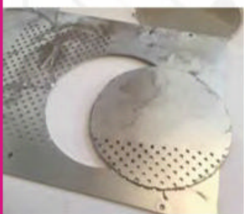
Adding a fan blowhole can boost cooling if you need to steal some of your case's ventilation for other features
