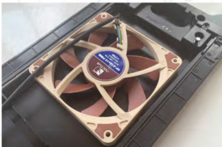
With the case on hand, I discovered that Noctua's new half-height fans could sit inside the side panel, allowing me to use more powerful components
