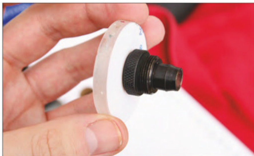
You can create threads for common PC screw sizes, and even G1/4in threads for water-cooling components
