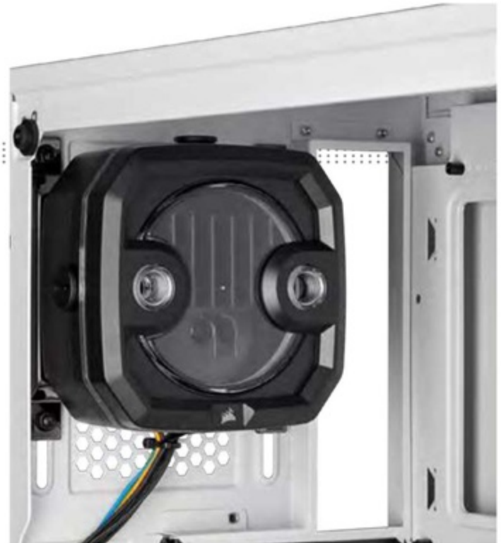
Corsair's new XD3 pump can fit into a 120mm fan mount
