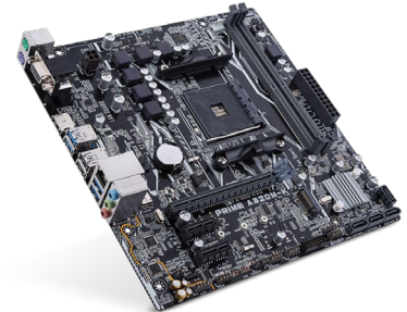
The Asus Prime A320M-K motherboard is a smaller microATX form so needs a smaller case
