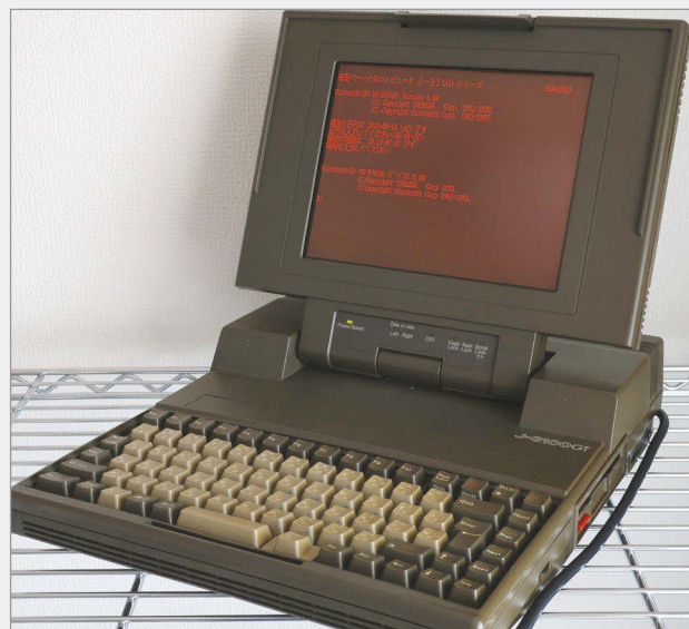
The Toshiba T3100, released in 1986, was a 'portable' PC that nevertheless relied on a mains power supply
