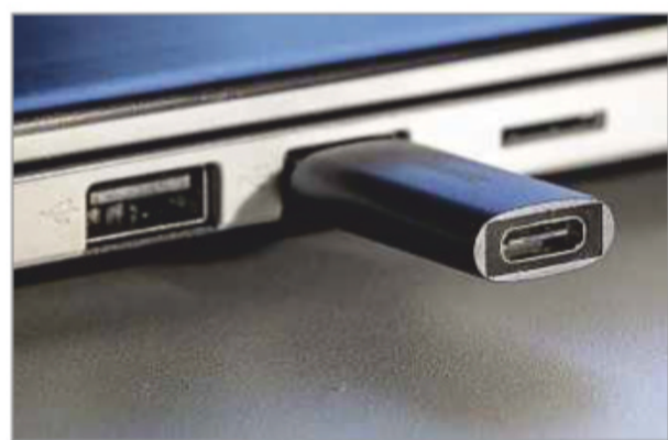
Buying an inexpensive adapter is a simple way to add USB-C support to your PC
