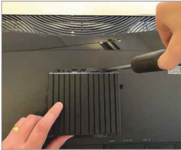
To create an all-in-one PC, screw the VESA mount attached to your mini PC into the rear of your monitor
