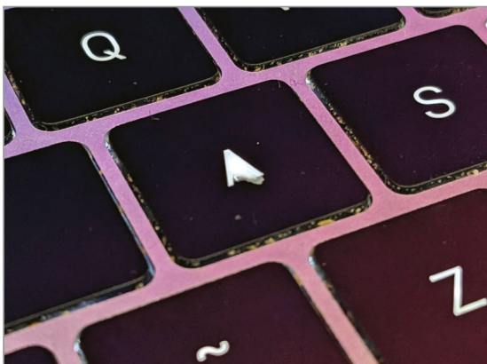
Some of the colour has rubbed off the 'A' key on this keyboard, allowing light to leak through
