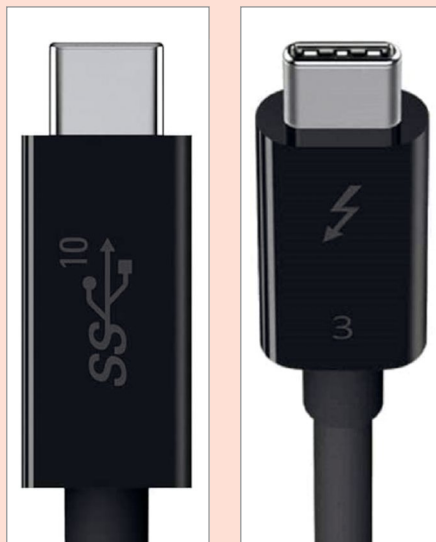
USB-C and Thunderbolt – the latest versions offer data-transfer speeds up to 40Gbps
