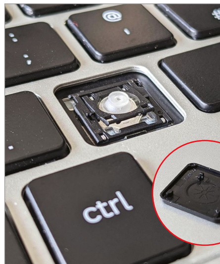
One of the keys has popped off our old laptop keyboard, but the mechanism still works
