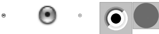
Figure 11.2 Radio buttons in Safari 5.0.1/OS X, Firefox 3.6.8/OS X, Firefox 3.0.1.5/Windows, IE 8/Windows, and Opera 10.6.1/Windows (from left to right) with a 100-pixel width, 100-pixel height, 1-pixel red border, and 10-pixel padding.
