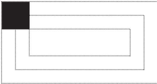
Figure 6.3 The position of the black #innerPositionedBox is measured from its containing block.
