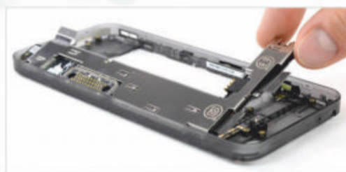
Removing the motherboard, we discover a bunch of spring contacts.
