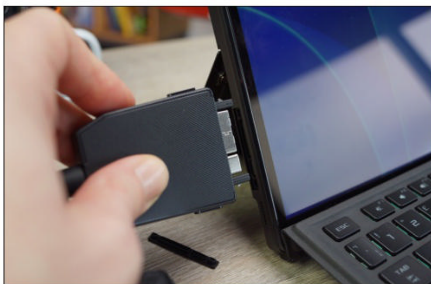
The XG Mobile connects to the Flow Z13 via a proprietary port on its left side.
