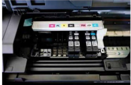
This illustration shows half the cartridges installed in an A3 8-ink printer.
