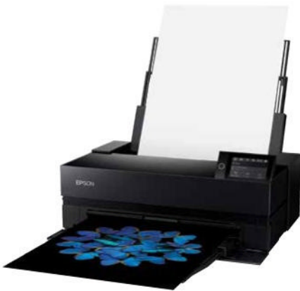
This A2 printer offers most of the capabilities professional users and serious enthusiasts require, including the ability to print on media up to 420 mm wide. Its 'footprint' measures 615 x 902 mm with output trays extended, as shown in this illustration. (Source: Epson.)
