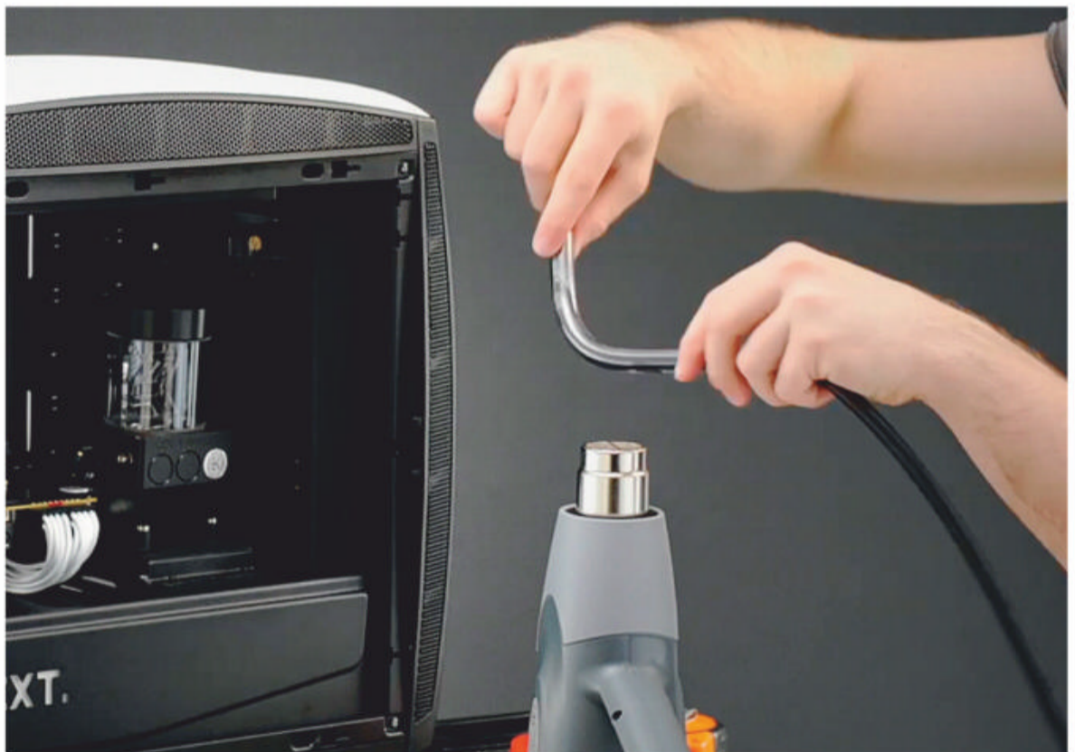
It's always smart to keep heating the outside edge while you perform the bend.
