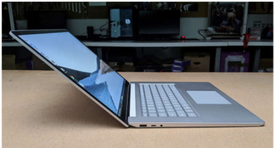
A USB-C port replaces miniDP in the latest iteration of the Surface Laptop, the Surface Laptop 3 for Business.
