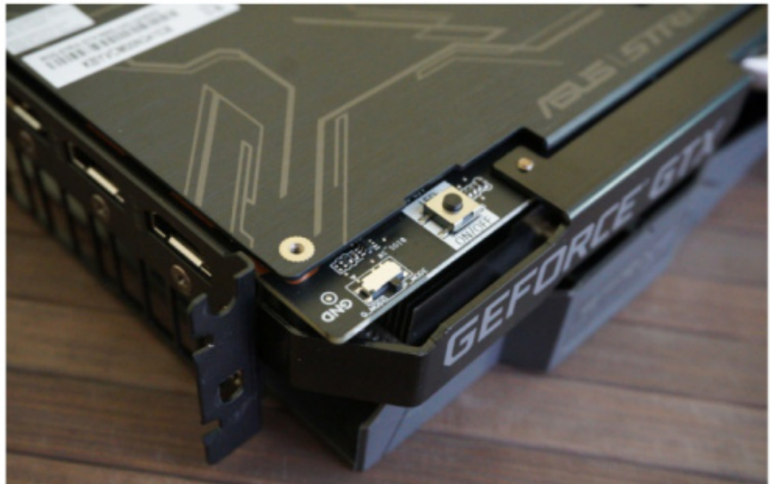
The Asus ROG Strix GTX 1650 Super's dual-BIOS switch.
