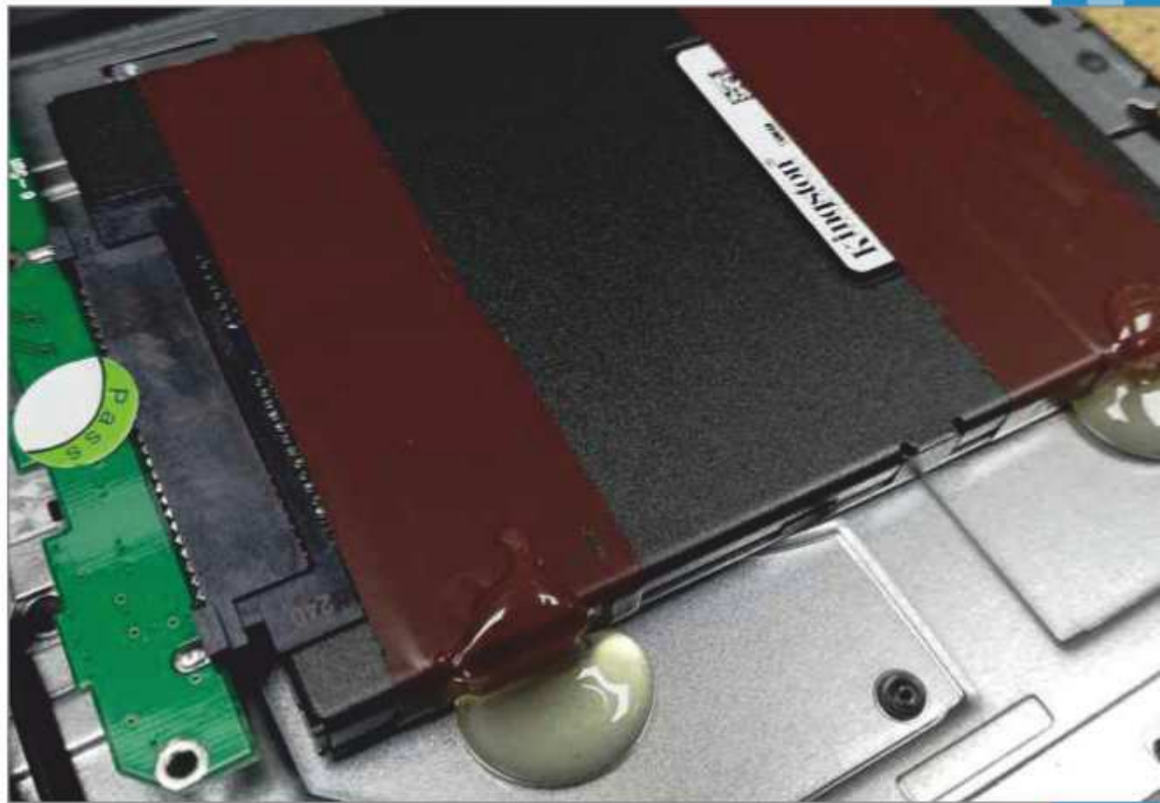
ABOVE I had to attach an SSD using the Blue Peter method – sticky-back plastic and a glue gun
