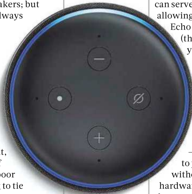
ABOVE You can no longer twist the top to change the volume, but the buttons are still there
