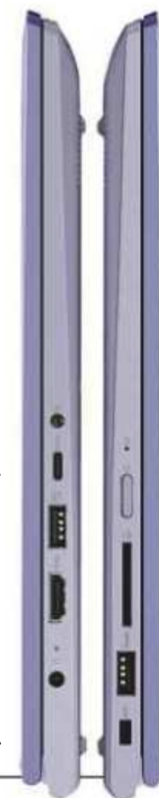
LEFT You're well served for ports: two USB-A, one USB-C, an HDMI slot and a 4-in-1 card reader
