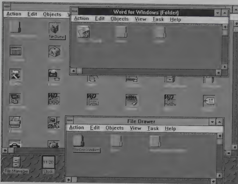
Figure 10.15 A folder can create programs, documents, and other folders. This folder contains a program and two additional folders.
