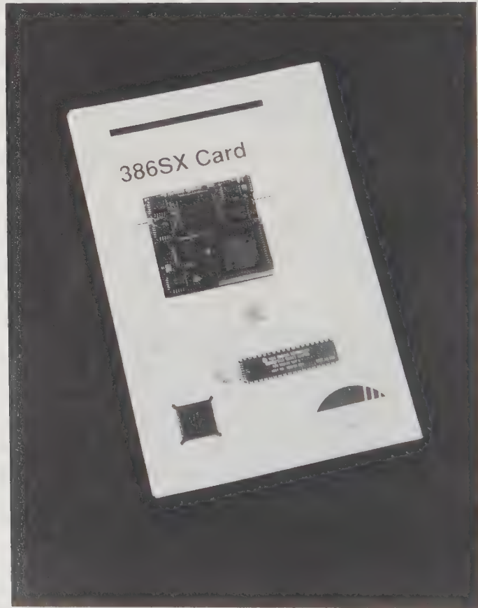
Figure 8-6. The Cumulus 386SX card (Photograph courtesy of Cumulus Corporation)
