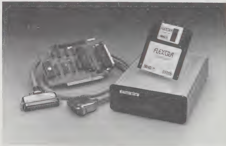
Figure 6-16. The Stor/Mor disk drive, media, and host adapter (Photograph courtesy of Q/Cor Corporation)
