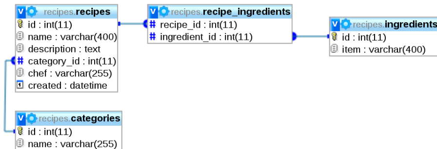
Figure 2.3. Our database schema with recipe_ingredients linking the recipes and ingredients tables
