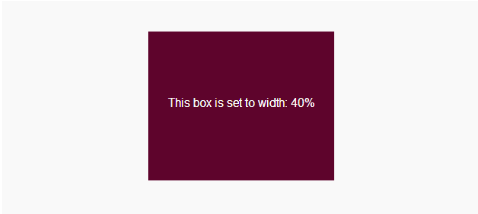
Figure 3.7. This box is set to width: 40%, making its width 40% of the available horizontal space in which it sits
