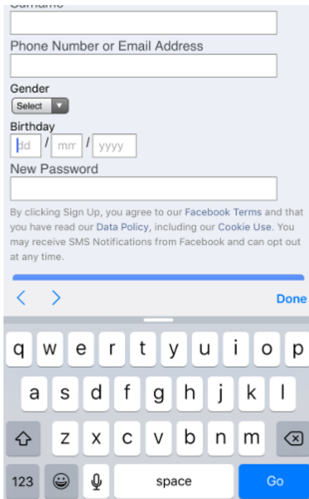
5-53. This birthday text box accepts only digits, but an alphabetic keyboard has come up
