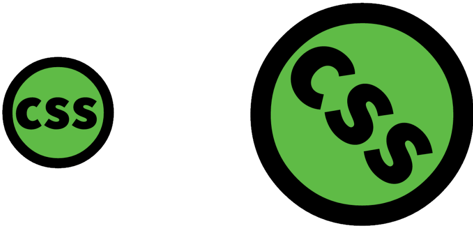
Figure 6.17. The original element (left) and after a combined rotation and scaling transformation is applied (right)
