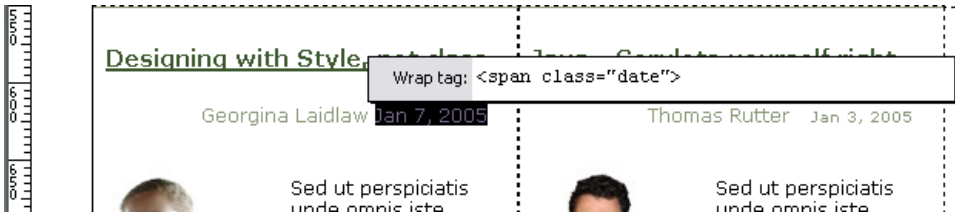
Figure 6.36. Using the Quick Tag Editor to add a span to the date.
