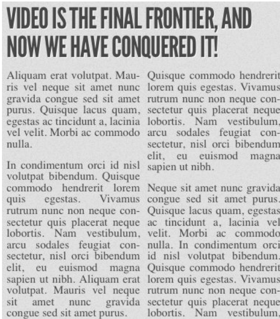
Figure 9.6. Declaring column-width in ems ensures a minimum number of characters on each line
