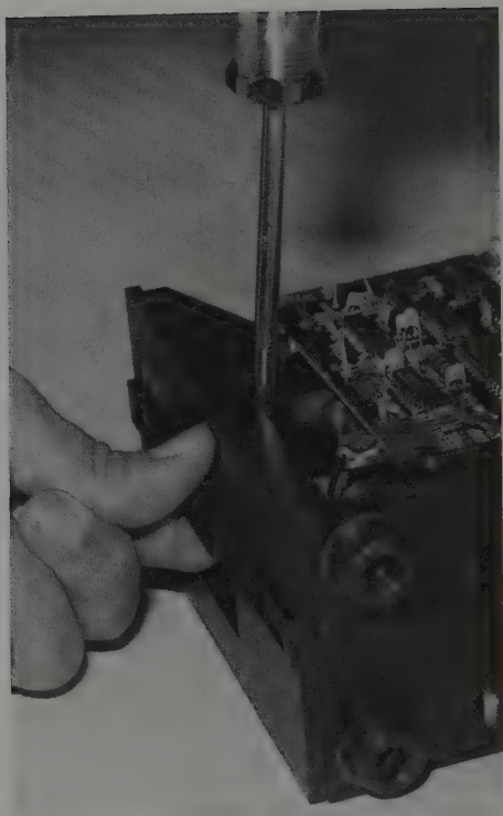
FIG. 4-7, 4-8 Replacing a door assembly.
