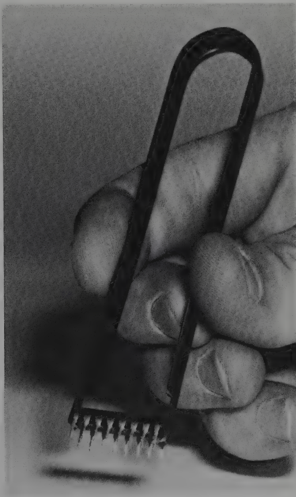
FIG. 1-4 The prongs of an IC are delicate, and the inside can be ruined by static. Handle with care!
