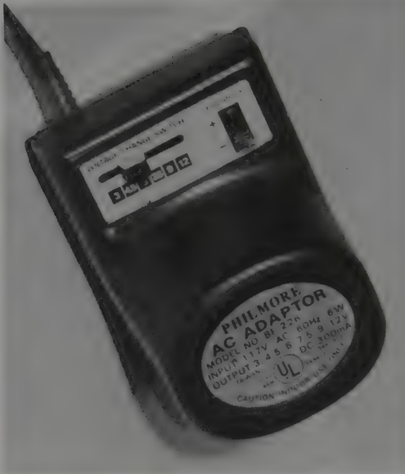
FIG. 6-3 Some small computers use an AC adaptor as a power supply.
