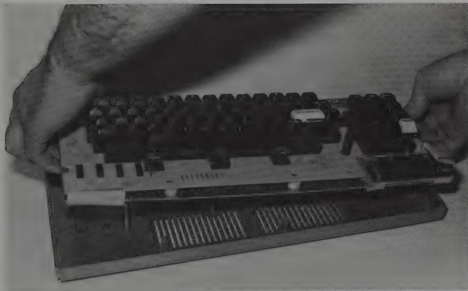
FIG. 5-6 Proceed carefully. In almost every computer made, if you've found all the holding screws and clips, the main board will lift out easily. Don't force anything.
