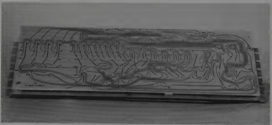
FIG. 6-13 The bottom of the circuit board. To replace a keyswitch, your first job will be to locate the two traces to that particular key.
